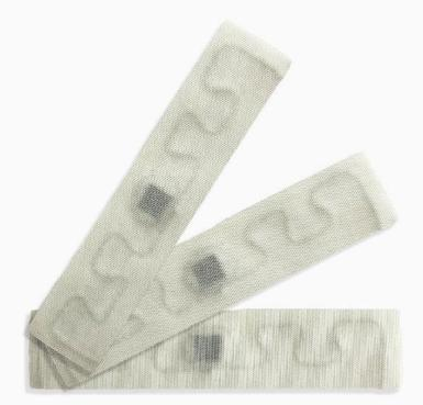
LT012 is a **fabric** RFID tag. Rectangular in shape, it is applied to the garment to be identified **by heat-sealing at 200°C, with a pressure of 2 Kg/cm2 for 30 seconds.**
