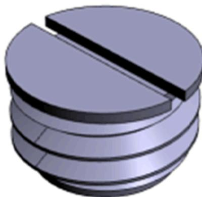
HT018 is an RFID hard tag made of Nylon, a plastic material resistant to impacts and atmospheric agents. Designed for **application on metal surfaces** using screws, it is cylindrical in shape, very light and very small. With a **diameter of 10 mm, it is 6 mm high and weighs just 0.33 grams**. It is available in black, and can be customised using laser printing.
