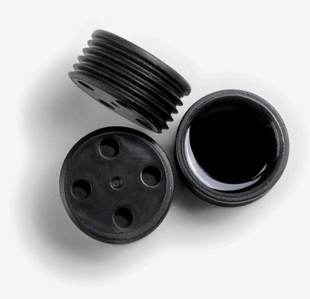
HT004 is an RFID bin tag made of PA6 (nylon), a plastic material resistant to tensile stress and compression, wear, and weather. The resin coating is made of PUR or polyurethane, which features good resistance to water, salt and moisture. Round in shape, the bin tag is designed for application on waste-collection bins. Its standard size — 30.5 mm in diameter — makes it easy to install and integrate into plastic containers.
