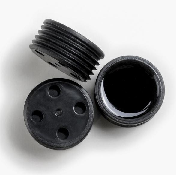
HT004 is an RFID bin tag made of PA6 (nylon), a plastic material resistant to tensile stress and compression, wear, and weather. The resin coating is made of PUR or polyurethane, which features good resistance to water, salt and moisture. Round in shape, the bin tag is designed for application on waste-collection bins. Its standard size — 30.5 mm in diameter — makes it easy to install and integrate into metal or plastic
