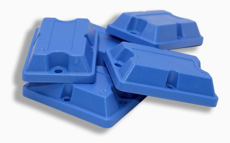
HT068 is an RFID hard tag made of polycarbonate (PC), a thermoplastic material with high resistance to temperature changes and fire, with elevated hardness and stress resistance. Rectangular in shape, HT068 weighs about 19 grams and measures 54 mm x 36 mm x 12.5
