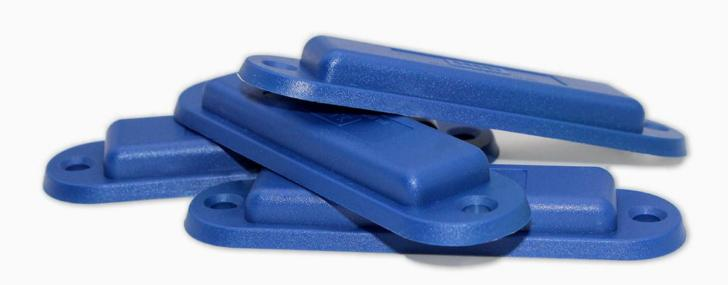
HT070 is a waterproof and extremely durable RFID hard tag in high-impact plastic that is resistant to impacts, cuts, high-pressure washing and high temperatures. Rectangular in shape, it weighs 15 grams and is available in two sizes — 97 mm x 27 mm x 15 mm and 97 mm x 27 mm x 10 mm. It allows for omnidirectional reading over long distances. The thinnest one — 10 mm — reaches 5 metres, while the thickest — 15 mm — reaches 8 metres. HT070 is configured for attachment via screws or welding
