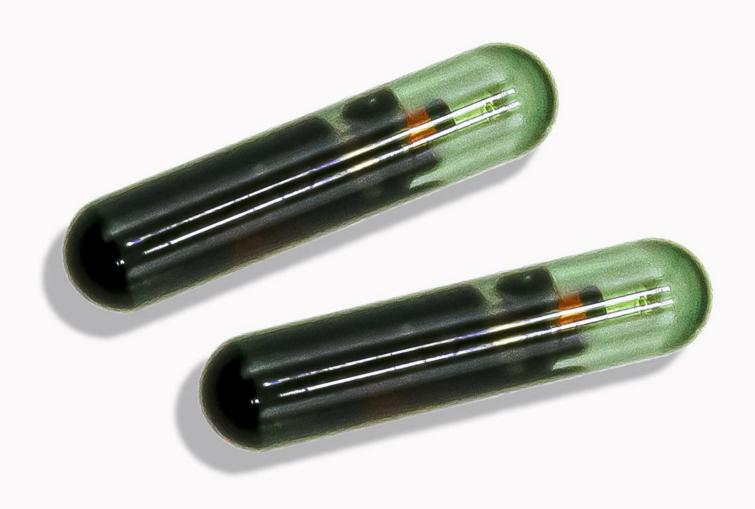
GT002 is a 'glass tag', thus made of glass, a transparent, chemically stable and versatile material. Cylindrical in shape, it is available in two sizes: Ø 2.12 mm x 12 mm and Ø 3 mm x 13 mm. This small size allows the tag to be easily embedded in any surface, whether metal or non-metal (plastic, wood, paper, water). Furthermore, the high resistance of glass protects the electronic components from exposure to aggressive chemicals,
