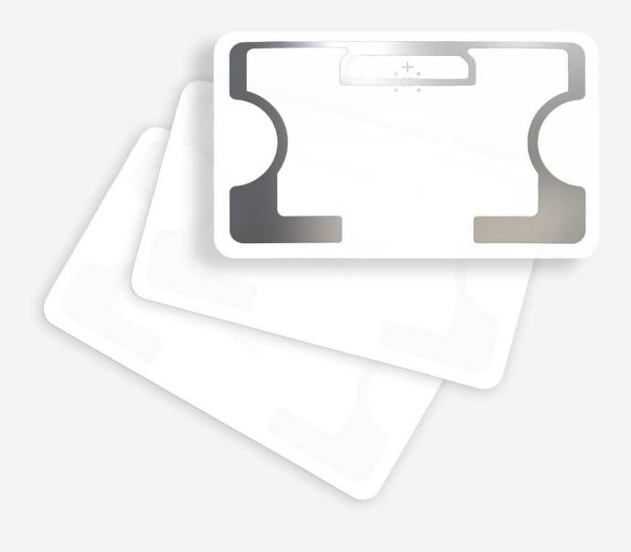
LB013 is a flexible and adhesive paper RFID label. Rectangular in shape, it measures 54 mm x 34 mm x 0.2 mm, while the **antenna inlay is 50 mm x 30 mm**. It is ideal for application **on non-metals** by means of an adhesive backing. It can be customised using offset or
