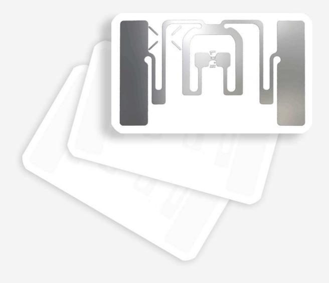
LB014 is an RFID label made of PET, a flexible, cut- and weather-resistant thermoplastic material. It is rectangular and measures 54 mm x 34 mm x 0.24 mm. LB014 can be applied to non-metal surfaces using a special adhesive. Printing and serial numbering are applied
