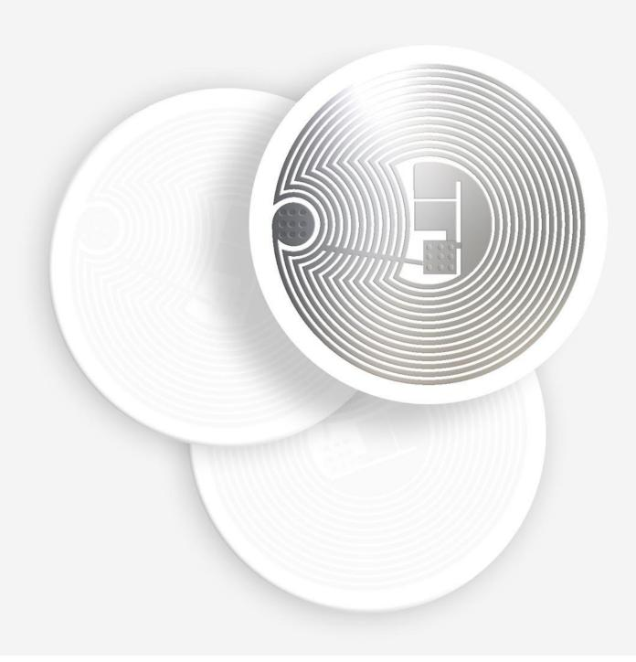
LB019 is a flexible and adhesive coated paper RFID label. Round in shape, it has a diameter of 30 mm, while the engraved aluminium inlay or antenna has a diameter of 27 mm. It can be applied to non-metal surfaces and is resistant to high
