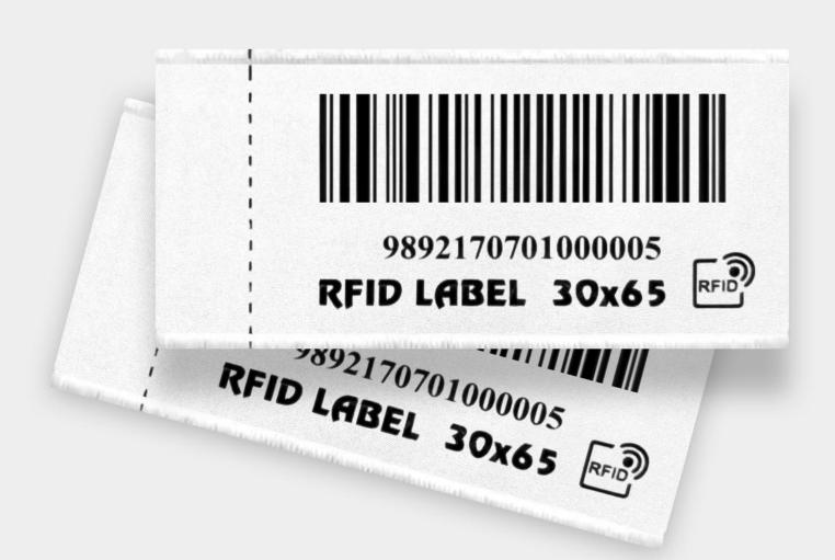
LT004 is an RFID label made of nylon taffeta, a smooth, soft and wear-resistant fabric. Rectangular in shape, it measures 30 mm x 65 mm, while the antenna housed in the fabric measures 15 mm x 40 mm. It is directly sewn into the
