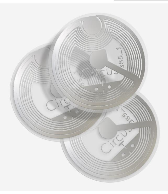
WT004 is a wet inlay made of PET, a flexible thermoplastic material resistant to cuts and thermal shock. Round in shape, it has a diameter of 22 mm and a thickness of 0.2 mm. It is transparent and is applied to non-metal surfaces by means of a special adhesive.
