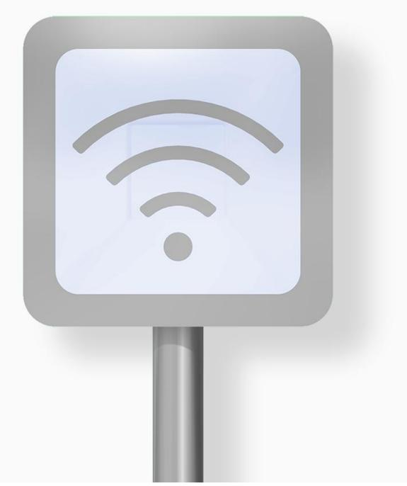
The Discovery Gate Light fixed RFID reader is a high power UHF device designed with **an external and an internal LED** for IoT applications.
