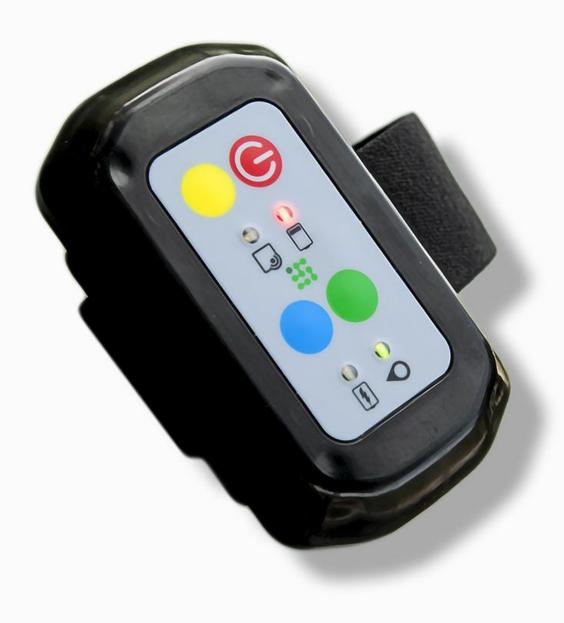
The Discovery Mobile UHF RFID wearable reader is a wearable device suitable for outdoor applications in dirty environments, due to its IP67 protection rating. This RFID wristband is ergonomic and particularly suitable door-to-door waste collection. It reads the RFID tag affixed on the bag or bin, records the deliveries per user, and transfers the data to the cloud via middleware at a user-defined frequency,
