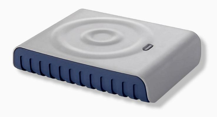
The D8 desktop RFID reader is a USB device operating in HF which detects HF RFID tags up to a distance of 10 cm. Easy to use and small in size — 122 mm x 93 mm x 25 mm — it is designed to read and write high-frequency RFID tags.
