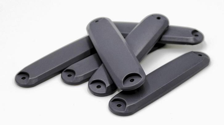
HT005 is a high performance, engineering plastic RFID hard tag that is resistant to mechanical stress, chemicals and high and low temperatures. Rectangular in shape, this tag measures 101.85 mm x 25 mm x 7 mm and can be applied to metal surfaces or other materials using screws or an adhesive backing. In particular, if the HT005 tag is affixed to metal, it can be read up to a distance of 5 metres, while if it is attached to plastic
