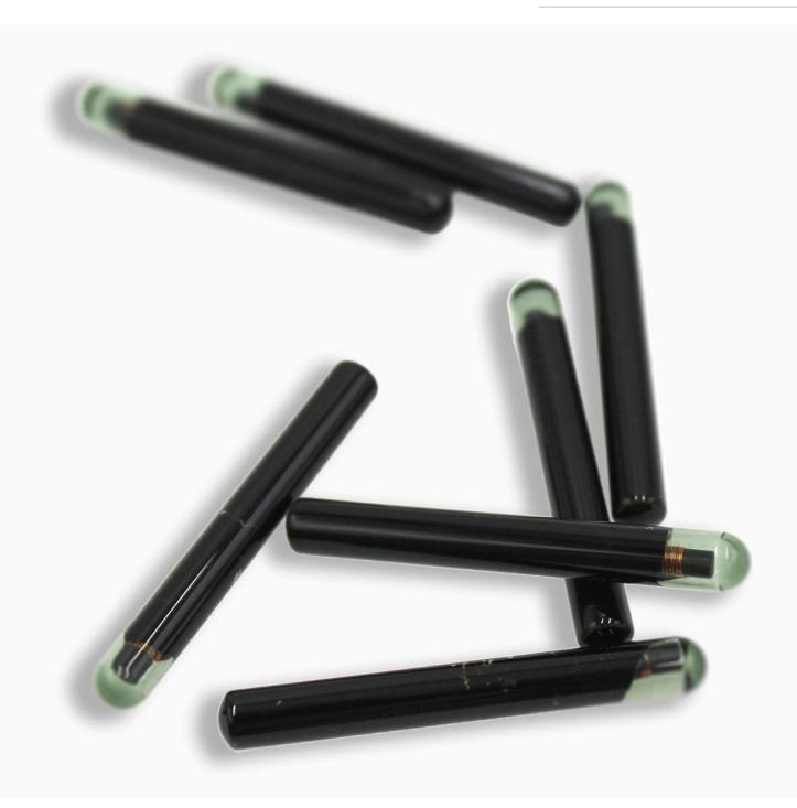
GT001 is a 'glass tag' made of biocompatible glass, a transparent, chemically stable and versatile material. Cylindrical in shape, it measures 3.85 mm x 32 mm. It is uniquely designed for the needs of any contactless RFID application in pet, farm and laboratory animal management. This glass tag can be applied via ingestion — it is housed inside a ceramic envelope that is
