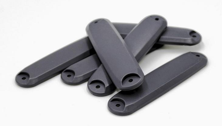
HT005 is a high performance, engineering plastic RFID hard tag that is resistant to mechanical stress, chemicals and high and low temperatures. Rectangular in shape, this tag measures 103 mm x 25 mm x 6.8 mm and can be applied to metal surfaces or other materials using screws or an adhesive backing. In particular, if the HT005 tag is affixed to metal, it can be read up to a distance of 5 metres, while if it is attached to plastic
