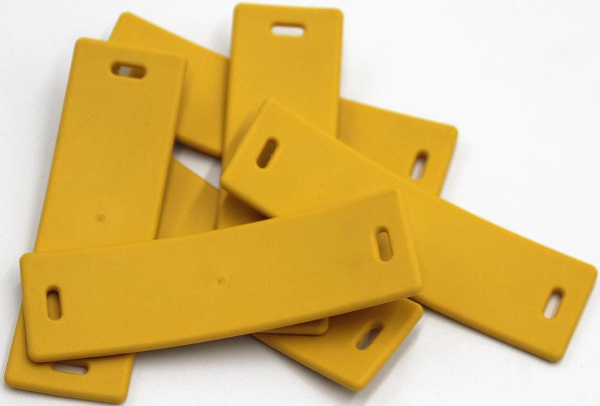
HT058 is an RFID hard tag made of **TPV (Vulcanised Thermoplastic), an elastomer combining the advantages of thermoplastic materials with those of rubber.** It retains good dimensional stability at high temperatures and is resistant to tensile stress and breakage, UV aging, ozone and weather. Rectangular in shape, it measures 83 mm x 26 mm x 2.6 mm and weighs 5 grams. **With its**
